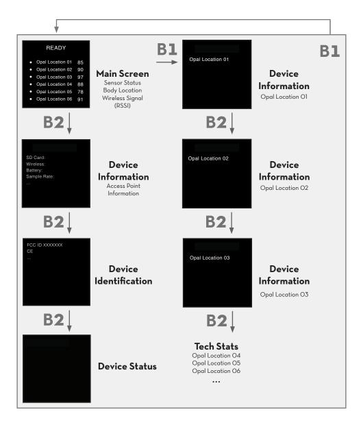
The Status screen on the AP indicates if the Opal sensors are ready to record data. Symbols on the left-hand side of the screen identify the following:
